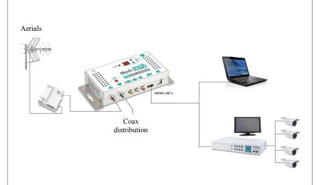
The **MOD-HDTV** the ideal solution for distributing HD or analog TV signals coming from e.g. a Audio/Video player, laptop or CCTV camera in a domestic coaxial network
