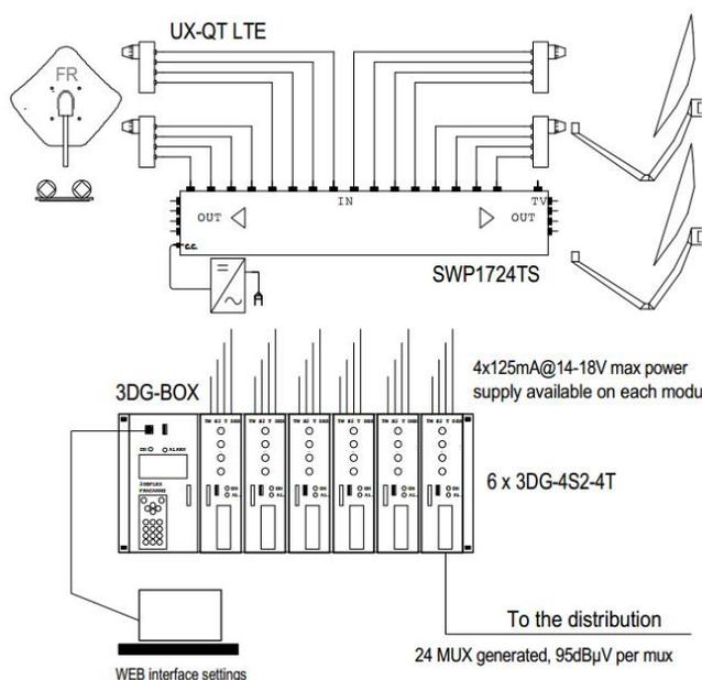
The new 3DG-4S2-4T quad transmodulator can tune up to four different SAT transponders, decrypt the programs (through CAMs & Smart-Cards – NOT INCLUDED) and generate four separate full-band RF Digital Multiplex (DVB-T or DVB-C), 95dBμV each.
