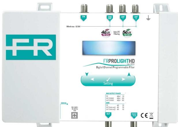
The Fracarro **FRPRO LIGHT HD** profiler is a flexible and programmable compact high-selectivity headend, equipped with an innovative technology, that allows to **filter, convert, amplify** and distribute many **DVB-T/T2** digital terrestrial multiplexes available in **VHF/UHF** band with the possibility to mix also the FM signal on the output distribution.
