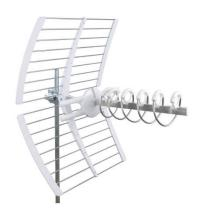
The Fracarro ELIKA LTE Aerials ELIKA series can be mounted on a pole without the need for tools thanks to its premounted elements, quick coupling radiator and reflectors, mast connector with standard zenith adjustment and large wingnut. These aerials benefit from a Built in 4G LTE Filter within the Dipole, high gain, excellent directivity and almost total absence of side lobes. Exclusive design patented by Fracarro.
